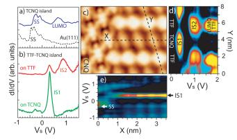
FIG. 2 (color online). Comparison of differential conductance spectra of (a) TCNQ pure islands [spectrum taken on a nearby clean Au(111) region shown for comparison] and (b) TTF and TCNQ in mixed TTF-TCNQ islands. (d),(e) The differential conductance spectra is mapped along the dashed lines shown in the STM image (c) ( $V_s = 1.9$  V;  $I_t = 0.07$  nA). The maps clearly show the spatial localization of IS1 and IS2 features on TCNQ and TTF rows, respectively.
