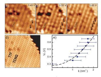
FIG. 3 (color online). (a)–(c) dI/dV maps of a TTF-TCNQ island, shown in (d), measured at the indicated sample bias values, lying above the onset of the IS1 resonance ( $I_t = 1.0 \text{ nA}$ ;  $16 \times 16 \text{ nm}^2$ ). (e) Dispersion relation E(k) obtained from data sets similar to (a)–(c). The dashed line is a parabolic fit to the data points, including the IS1 peak position.
