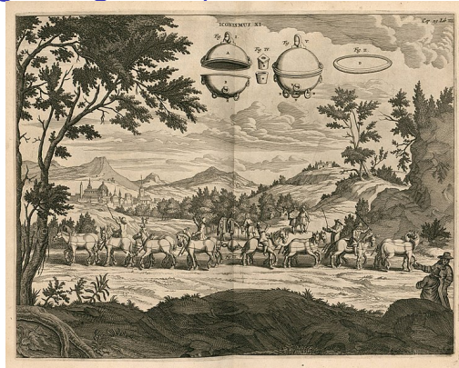
The Magdeburg hemispheres (1654) — a tool to demonstrate the force of atmospheric pressure — empirical proof of the existence of vacuum
