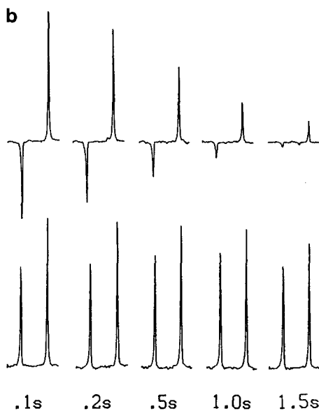
FIG. 6. Laboratory-frame ^{15}\text{N} CPMAS polarization-transfer experiment on TTP at 6.082 MHz and -88^\circ\text{C} using pulse sequence A. CP time 25 ms, 3000 scans per spectrum, 1.2 s repetition time, 2.4 kHz sweep width. (b) top: experiment II with t_1 = 761 \mu\text{s} ; (b) bottom: experiment I with t_1 = 0 ; (a): nonlinear least-squares data fit using Eq. [3]. The polarization transfer arises again (see Fig. 5) mainly from spin diffusion.
