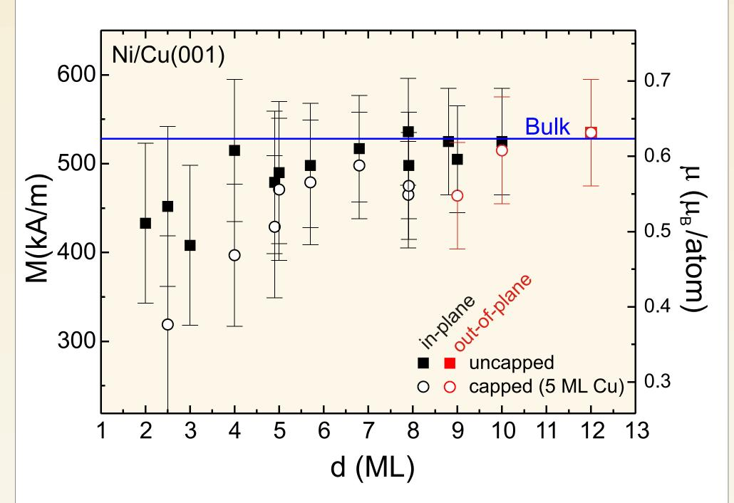
The measured remanent magnetizations at 40 K were extrapolated to T=0K. A series of Ni/Cu(001) films between 2 and 12 ML is shown before ( $\blacksquare$ , $\blacksquare$ ) and after ( $\bigcirc$ , $\bigcirc$ ) Cu capping.
