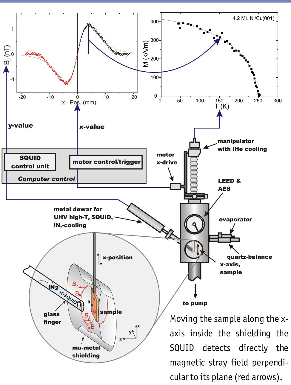
This stray field is recorded as a function of space. The upper-left graph shows such a single measurement of an in-plane magnetized sample.
