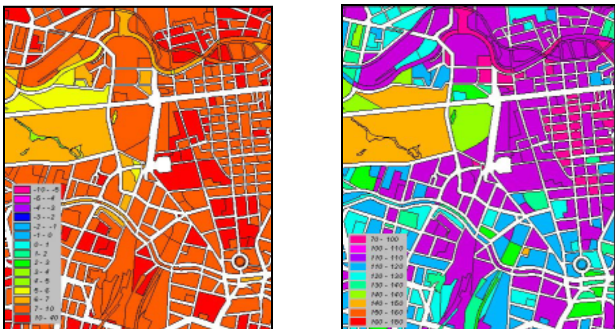
Fig. 4: Day-night-difference of surface temperatures and NDVI related to urban structure polygons, example “Potsdamer Platz”; a) day-night-difference 14.08.00/13.08.00 in Kelvin; b) NDVI extracted from ETM+ in DN calculated with following term ((B4-B3)/(B4+B3)+1)*127
