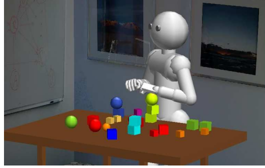
Figure 4.12: Clearance task with relevance grounding. The robot has to clear up the desktop by piling objects of the same size and color. Focusing on relevant objects permits efficient reasoning in this scenario containing many objects.
