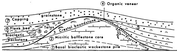
Figure 10 Ideal carbonate mud mound with seven commonly developed facies units. The sequence of facies develops when the mound grows into the wave base.
