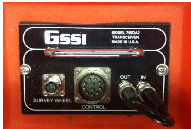
Figure 1: Model 769DA2 Transceiver (with co-axial jumper inserted for mono-static mode).
