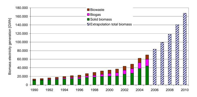
Figure 6: Historical development of electricity generation from solid biomass, biogas and municipal solid waste in the EU-25 Member States from 1990 to 2004 and extrapolation to 2010 assuming a yearly growth rate of 19%<sup>23</sup>.
