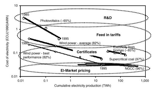
Fig. 4. Complementary support systems imposed on IEA's learning curve estimates. (Source: From IEA (2000)).
