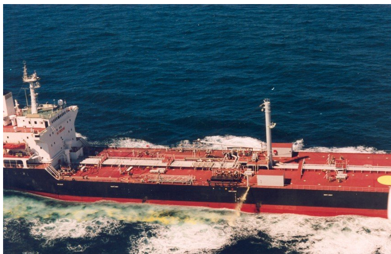
Picture 1: Discharge of white oils form tankship in the North Sea - legal at that time (photograph from surveillance plan kindly provided by the Netherlands' Ministerie van Verkeer en Waterstraat, Directorate-Generaal Goederenvervoer, Den Hague)
